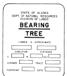
TYPICAL 4 1/2" x 6" BEARING TREE TAG
