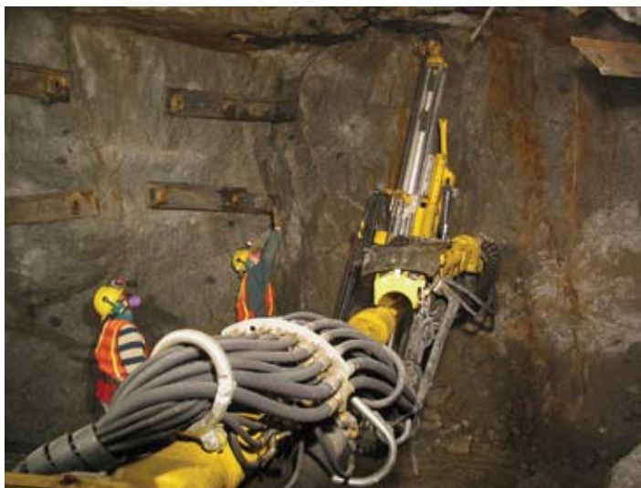
Student miners Nikoly Zarembo and Viktor Fendich work with a jumbo rock drill as they learn ground control, the process of securing the mine shaft to make a safe work area. The two students are at the Delta Mine Training Center (DMTC) in Delta Junction. Photo courtesy of DMTC.
