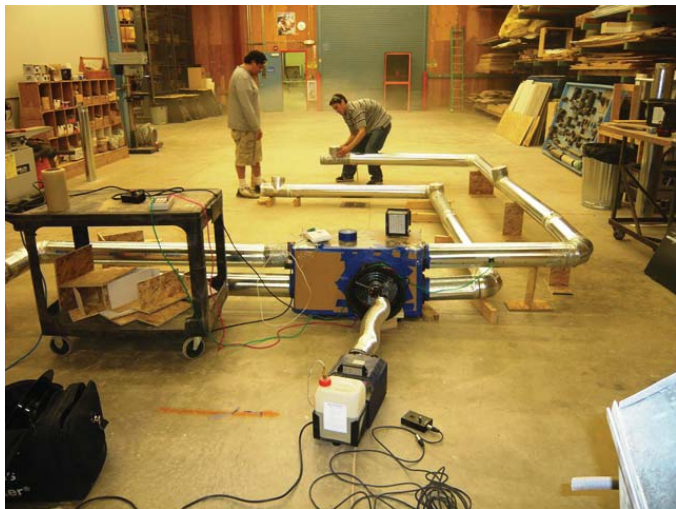
Photo 3.36 TEC Construction Technology - Blower Door Testing
