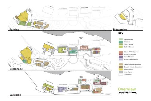
**Project Description:** Renewal of the Whitehead and Hendrickson Buildings including replacement of heating, ventilation, lighting and electrical distribution systems. Building envelopes will be significantly improved to reduce energy consumption. Work will include relocations of current occupants and work outside of these two buildings that is required to accommodate tenant relocations.
