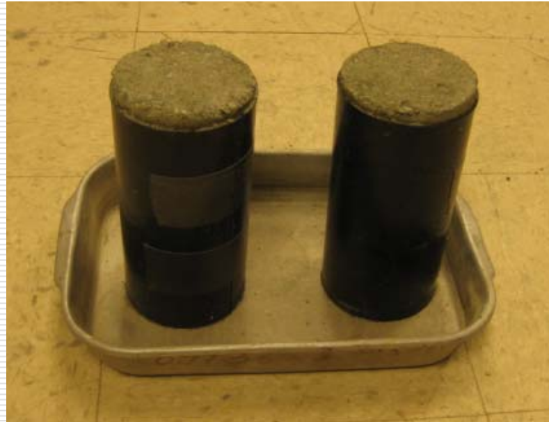
Soil samples after frost heave test
